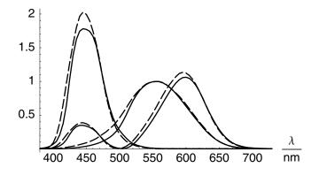
Figure 2: Color matching functions. Solid lines =  $2^{\circ}$  observer; dashed lines =  $10^{\circ}$  observer
